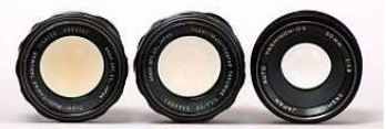
Yellowed thorium dioxide lens (left), a similar lens partially de-yellowed with ultraviolet radiation (centre), and lens without yellowing (right)
