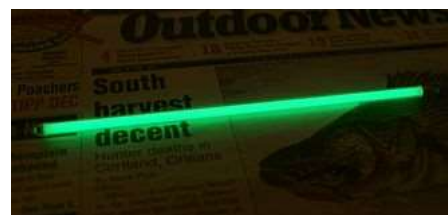
Radioluminescent 1.8 curies (67 GBq) 6 by 0.2 inches (152.4 mm × 5.1 mm) tritium vials are thin, tritium-gas-filled glass vials whose inner surfaces are coated with a phosphor . The vial shown here is brand-new.
